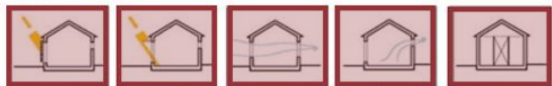
C1 window shutters C2 sun shading elements C3 cross ventilation C4 stack effect C5 semi-open space (portico)
